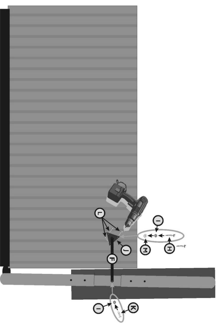
Use the power screwdriver to secure the Chain Mounting Bracket **J** to the spa cabinet with the small Wood Screws **L**. The other end of the chain is secured to the Side Arm with a small Machine Screw **K** and #10 Flat Washer **I**.
