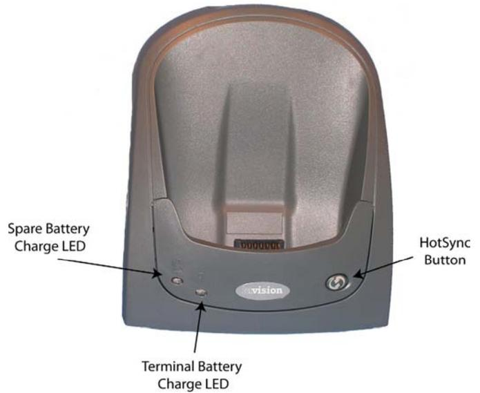
A switch on the back of the cradle controls which type of sync the cradle is to perform. With customized or third party software, it can also be used to synchronize your SPT 1700 or SPT 1800 terminal with corporate databases and other host computers.
