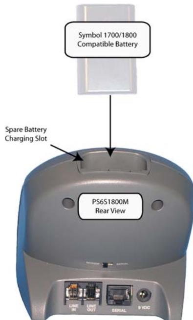
To charge the terminal's spare battery:
